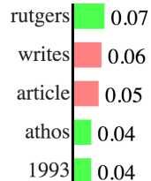
Figure 1: Explaining a document classification prediction (logistic regression on 20 Newsgroups, K = 5 ). The classifier correctly predicts the class 'Christianity' with p = 0.59 . In the explanation, words indicative (according to the model) of 'Christianity' are green, while 'Atheism' words are red.
